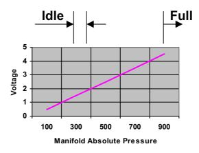
() When the SGI system is used in engines equipped with boost pressure (turbo), the reach of the MAP sensor integrated into the Interface Unit is not sufficient. In that case the original MAP sensor of the engine concerned must be branched off. In case the engine-management system is not fitted with a MAP sensor, a separate MAP sensor will be included in the SGI engine kit. Both situations are clearly explained in this installation manual.
