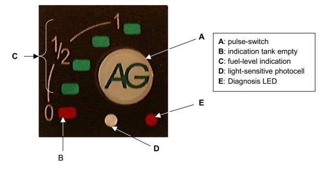
**A** is the switch to change over from LPG to petrol. Because it is a pulse switch, it only needs to be touched slightly to switch between petrol and LPG.
