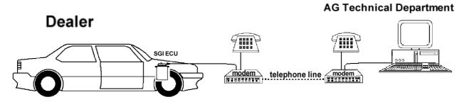
When all the necessary connections have been made, the switch should be set to LPG and the ignition <u>off</u>. Then the so-called modem line (see appendix) can be contacted, using the telephone in the test kit.
