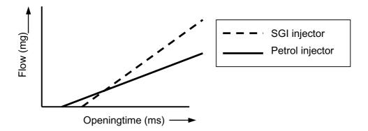
To be able to measure the opening period of the petrol injectors, they are simulated by the interface unit when driving on LPG. This simulation signal communicates the opening periods separately to the SGI computer. The computer then converts these periods to the exact opening periods for each SGI injector separately.
