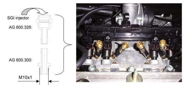
The length of the LPG hose between the SGI vaporiser and the Fuel Rail is not really important for the performance of the system (it is a good starting point to keep it as short as possible).
