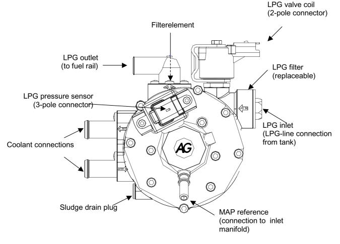
The absolute pressure in the vaporiser is gauged by means of a pressure sensor, so that the SGI system does not suffer any adverse effects from pressure fluctuations in the vaporiser. The absolute pressure varies between 950 mb. (when decelerating) and 1800 mb. (at full load).
