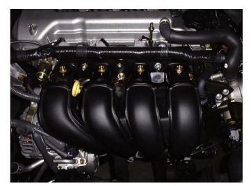
AG 600.300 in combination with AG 600.326, to fit the SGI injectors indirectly into the inlet manifold by means of an 8 mm hose (see photographs below). These nipples are used when the injectors cannot be fitted sufficiently close to the inlet with the standard nipples.
