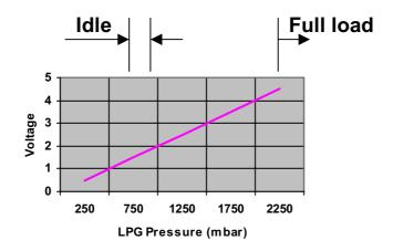
The differential pressure across the SGI injectors is equal to the difference between the pressure measured in the inlet manifold and the LPG pressure in the vaporiser. Any variation in the differential pressure can be corrected by means of the software.
