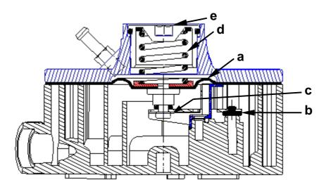
As shown, underneath the membrane (a) LPG is allowed to enter the vaporiser along the valve (b), which is fitted onto the lever (c); when the shut-off valve is open.
